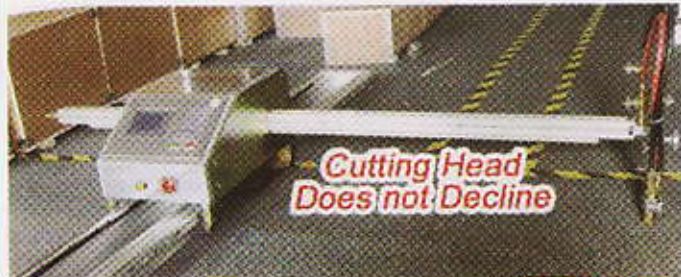
Guiding System of the Cross Beam
