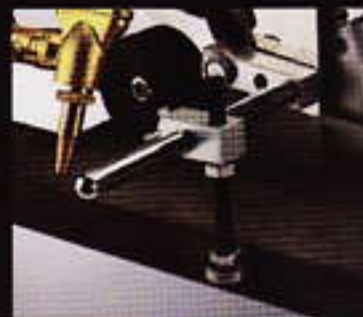
Tracer guide roller
